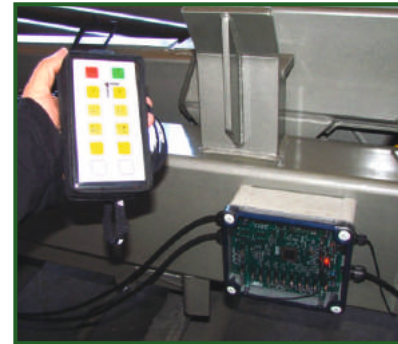
STR-705 Two pipes to the tractor hydraulic system with distributor operated by remote control.
