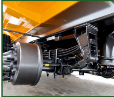
STR-407 32t parabolic sprung suspension, 1810mm distance between axles.
