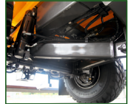
STR-410 Hydraulic suspension for optimal axle travel.
