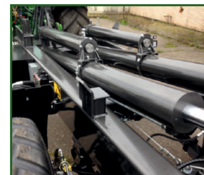
STR-1005 PowerBoosta™ – pair of booster cylinders, increasing tipping and unloading cycle power.
