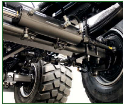
STR-214 CommandSteer™ - in-cab control – excellent manoeuvrability in reverse – free steering travelling forwards. Only on rear axle.
