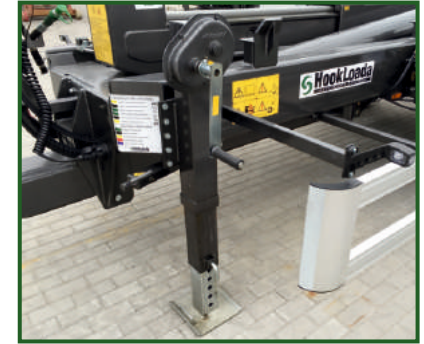
Stabilising legs available: • Manual geared telescopic leg • Manual telescopic support leg • Suspended shoe-type leg
