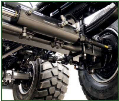
STR-214 CommandSteer™ - in-cab control – excellent manoeuvrability in reverse – free steering travelling forwards.
