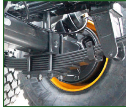
Suspensions available: • Multileaf sprung suspension • Parabolic sprung suspension
