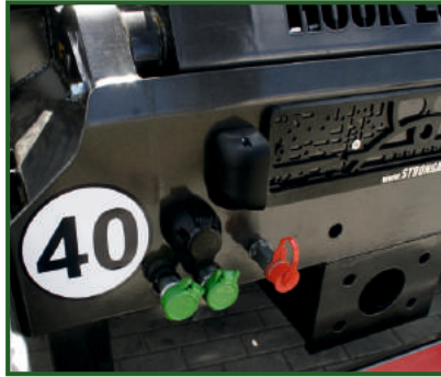
STR-1038 Rear mounted hydraulic brake connection.
