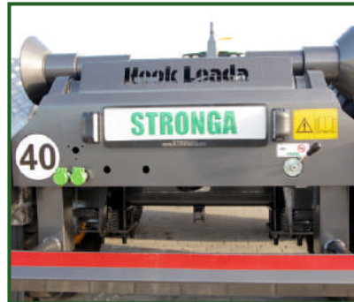
STR-700 Auxiliary hydraulic connections with changeover valve at the rear of the trailer.
