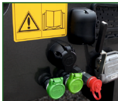
STR-1039 Rear mounted light connection 7-pin socket.
