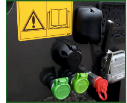
STR-1039 Rear mounted light connection 7-pin socket.
