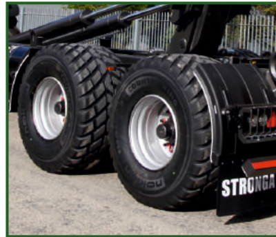
STR-903 Hard plastic quarter mudguards, front and rear.
