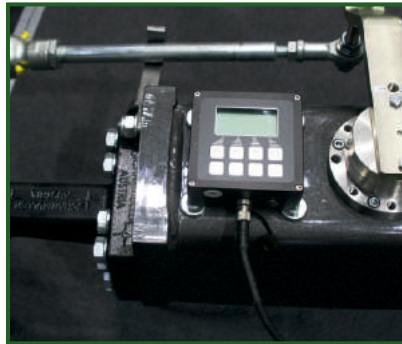
STR-707 Electronic Power Steering (EPS).
