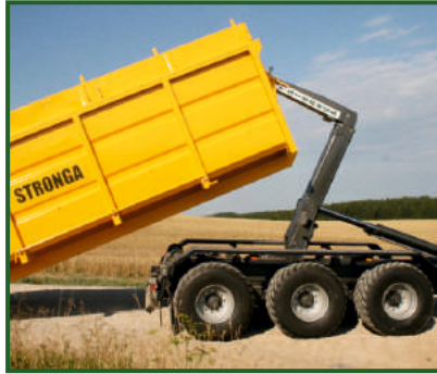
STR-713 QuickLoada™ fast tipping and unloading system.
