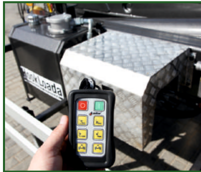
STR-704 Independent hydraulic system with PTO. Distributor operated by remote control.
