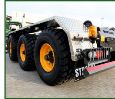
STR-900 Full length ultra-light aluminium mudguards.
