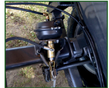
STR-305 Dual air and hydraulic brake system.
