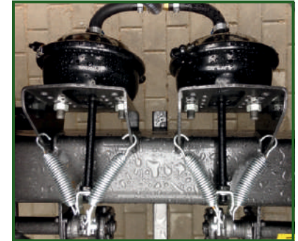
Brakes available: • Air brakes on all wheels (excl. Load Sensing Valve) • Hydraulic brakes on all wheels
