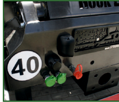
STR-1038 Rear mounted hydraulic brake connection.
