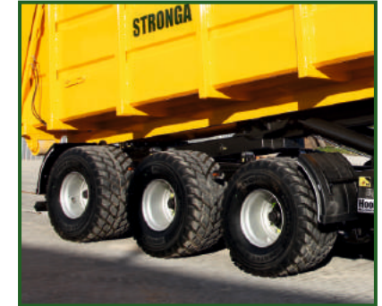
STR-903 Hard plastic quarter mudguards, front and rear.
