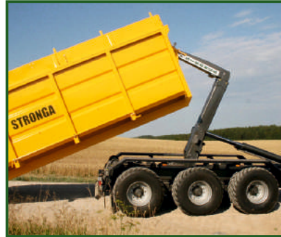
STR-713 QuickLoada™ fast tipping and unloading system.
