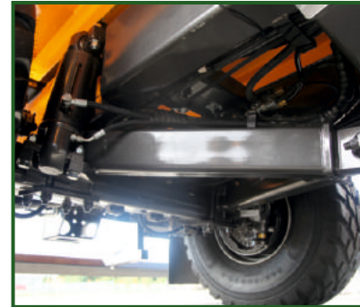
STR-410 Hydraulic suspension for optimal axle travel.
