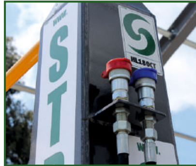
STR-710 Auxiliary connections on the hook tower with changeover valve.
