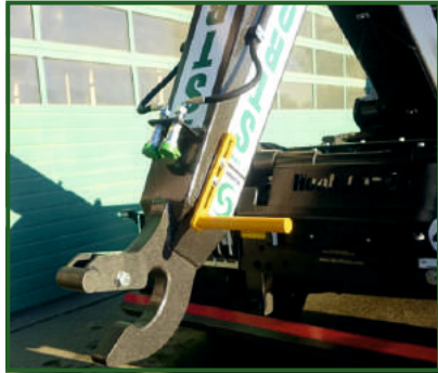
STR-724 Auxiliary connections with electrical changeover valve on the hook tower.
