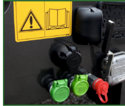
STR-1039 Rear mounted light connection 7-pin socket.
