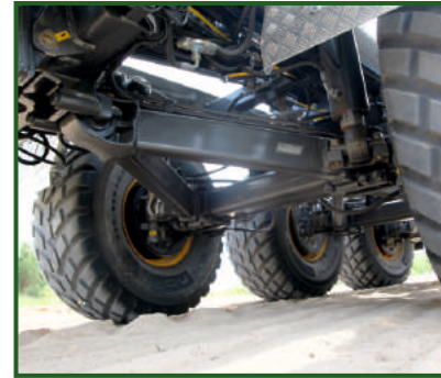
STR-410 Hydraulic suspension for optimal axle travel.
