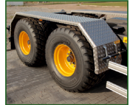
STR-900 Full length ultra-light aluminium mudguards.
