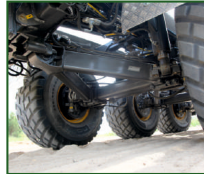
STR-410 Hydraulic suspension for optimal axle travel.
