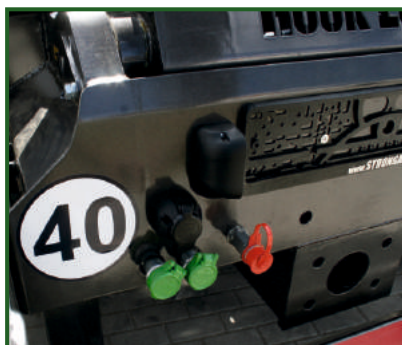
STR-1038 Rear mounted hydraulic brake connection.
