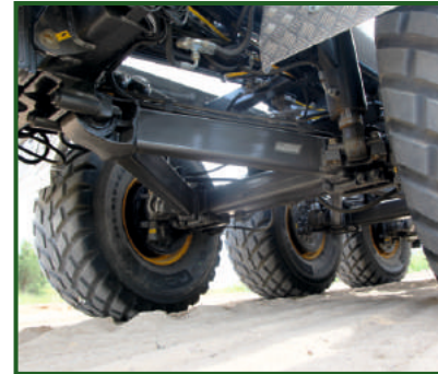
STR-410 Hydraulic suspension for optimal axle travel.
