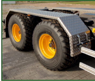
STR-900 Full length ultra-light aluminium mudguards.
