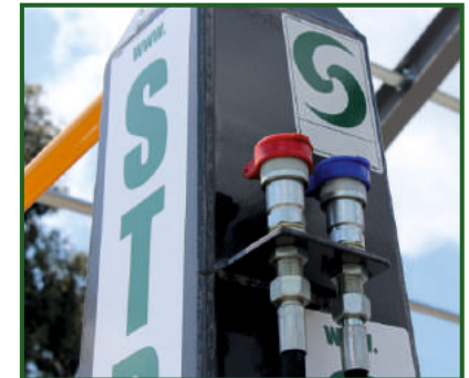
STR-710 Auxiliary connections on the hook tower with changeover valve.
