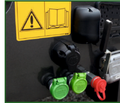
STR-1039 Rear mounted light connection 7- pin socket.
