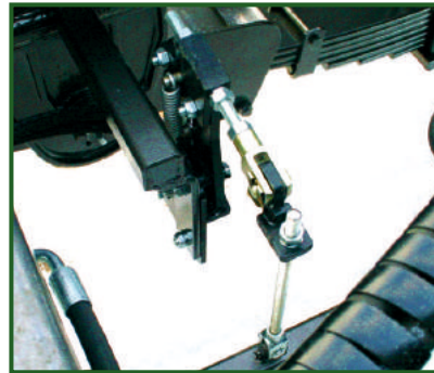
STR-302 Load sensing for hydraulic brakes.
