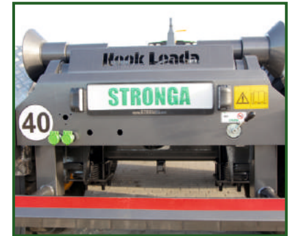
STR-700 Auxiliary hydraulic connections with changeover valve at the rear of the trailer.
