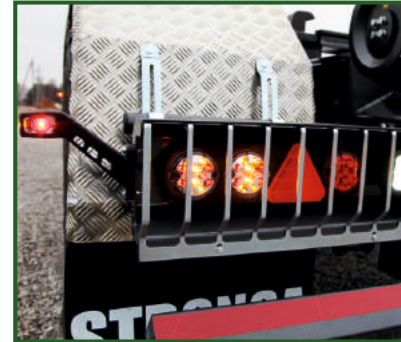
12 V electric system. Sealed loom. All lights super-bright LED.
