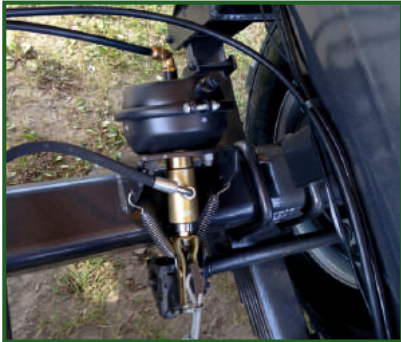
STR-305 Dual air and hydraulic brake system.
