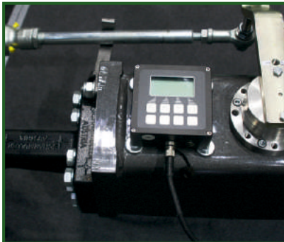
STR-707 Electronic Power Steering (EPS).
