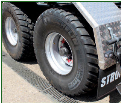
560/60 R22,5 Michelin Ultraflex radial tyres. 10 stud heavy-duty wheels.
